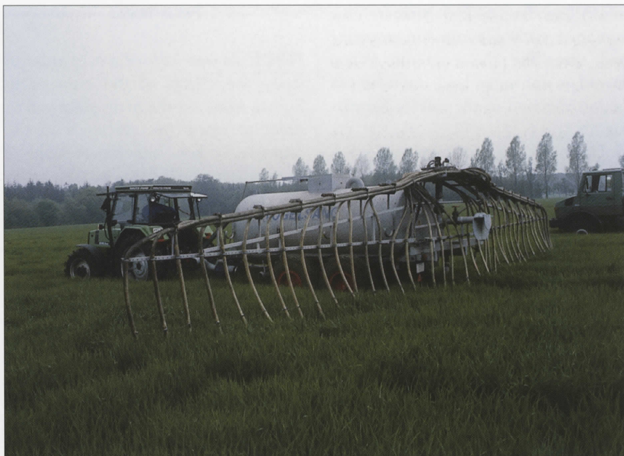
Tank wagon with an applicator fitted with trailing hoses. The fertilizer is usually fed to the hoses through a centrally located distributor.
